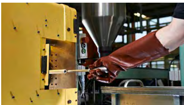
Manufacture of the inner tube reinforced with metal core for plastic versions.
