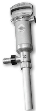
The worldwide first electrical drum pump
