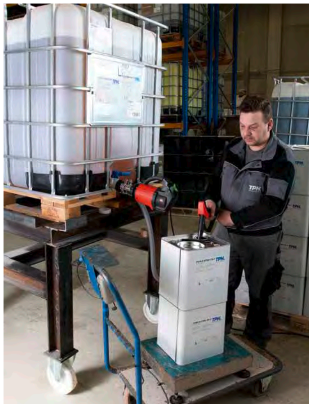
Fast container filling from the IBC outlet.
